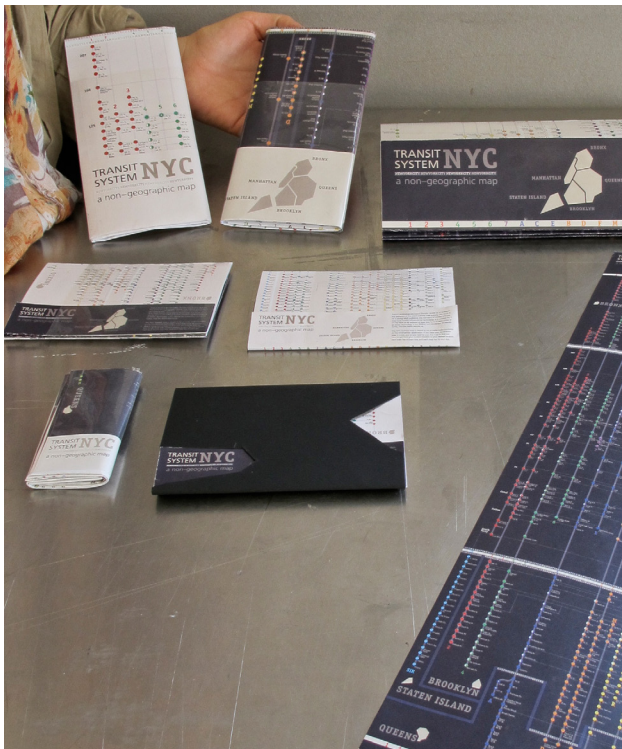
FIGURE 8: In order to test the practicality of the design a complete set of comprehensives were printed and folded to the correct size. These prototype comprehensives permitted final analysis and critique of program detail, such as aspects of editorial clarity and readability.
